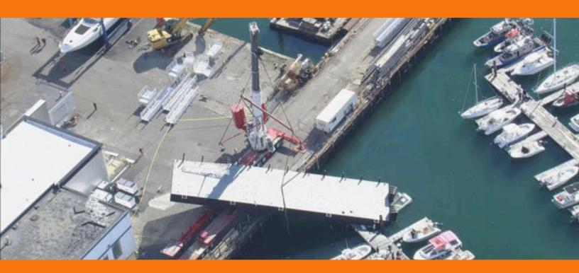
The Boston Fire Department told WBZ-TV the crane was putting up a barge around 11 a.m. when the rigging suddenly snapped. The barge crushed part of a dock and a boat as it fell into the water. Witnesses said the impact shook the ground beneath them and startled those working nearby Click here to read the full article.
